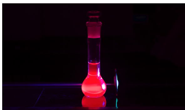
The europium Eu(III) complex with nanocarbon antenna emitting fine red light.
